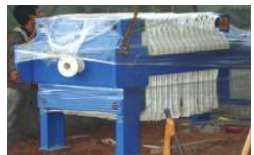
Sludge Handling (Filter Press)
