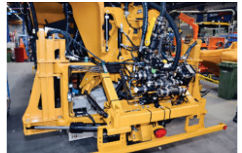
Special hydraulic hoses and piping
